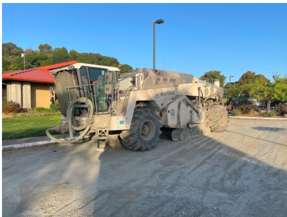
Photo 7: Cement base treatment equipment used for mixing subsoil.
