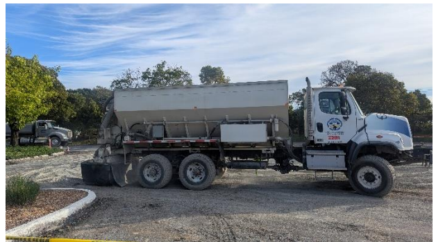
Photo 6: Cement base treatment equipment used for spreading cement.
